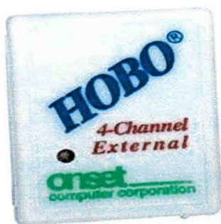
Figura 6. HOB0 4- Channel (datalogger )
