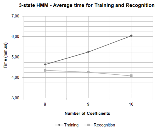
Fig. 7. Relationship between training and recognition time and the number of coefficients for 3-state HMM.
