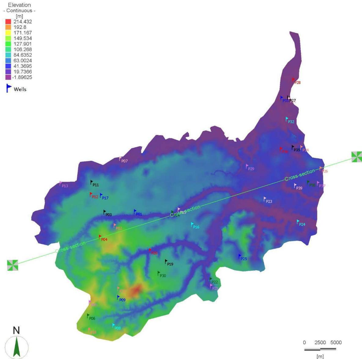
Figure 4.3 - Numerical model topography and location of the phreatic wells (colors are for differentiation)
