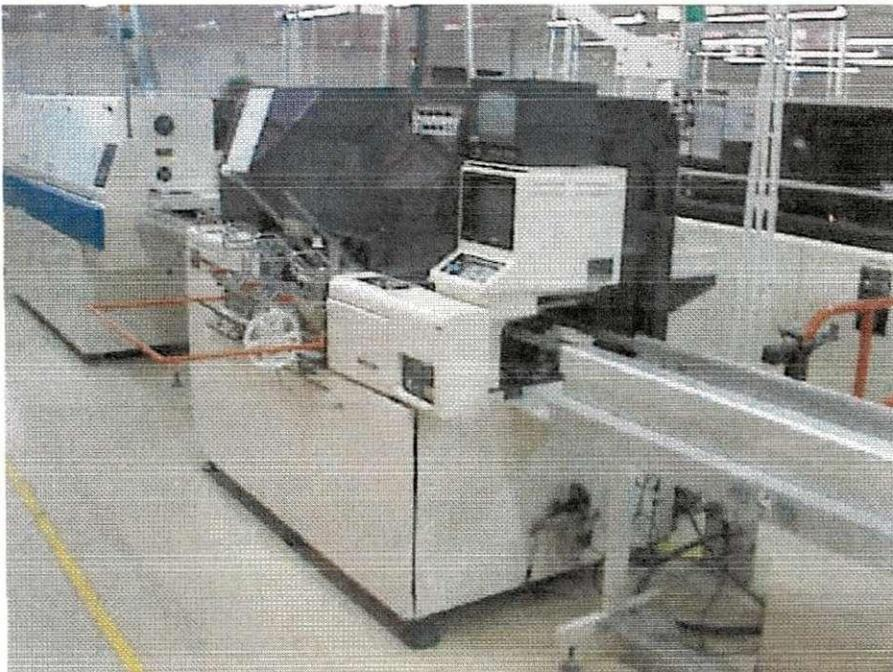
FIG. 12: MPA (AO CENTRO) SEGUIDO DO FORNO (À CIMA E À ESQUERDA)
