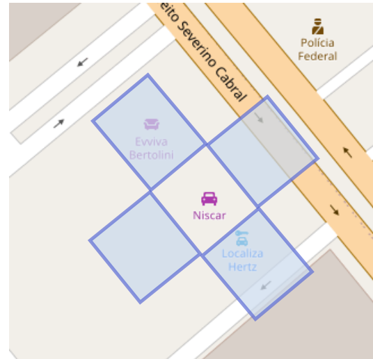
Figure 14: One-sided buffer, computed for each of the sides of the landmark polygon.
