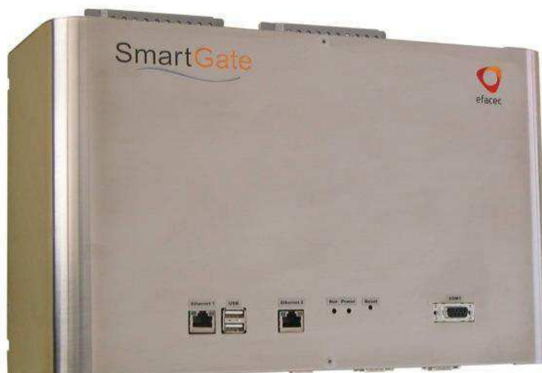
Figura 12 – Smart Controller/Meter Concentrator – EFACEC [12].
