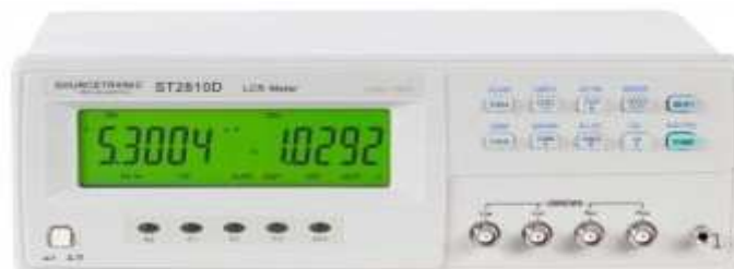
Figura 31 - Sourcetric LCR Meter 2810D
