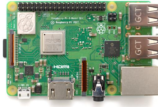
Figura 9 – Raspberry Pi 3 Model B
