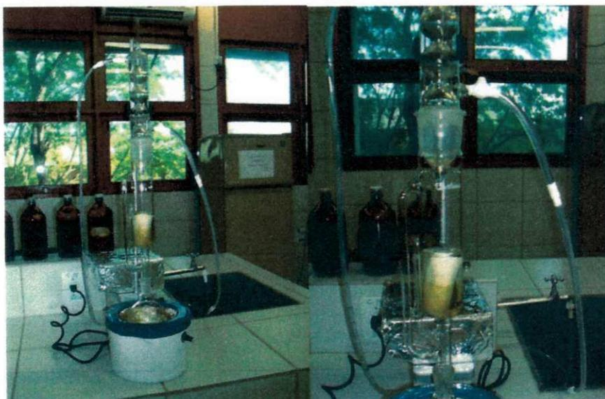
Figura 10: Extrator Soxhlet
