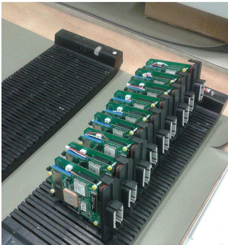
FIGURA 3 – PCBs FABRICADOS PARA MONTAGEM DO PRODUTO FINAL.
