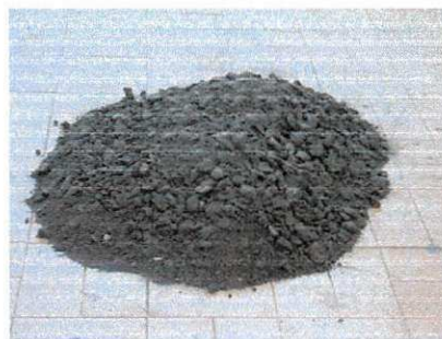
Figura 33: Material fresado passado na peneira 3/4"
