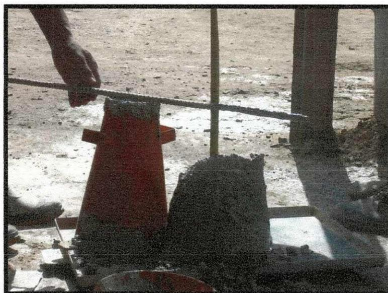
**Figura 32 Slump test.**
