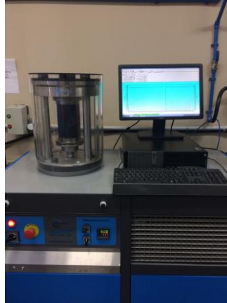
Figura 25 - Asphalt Mixture Performance Tester (AMPT)
