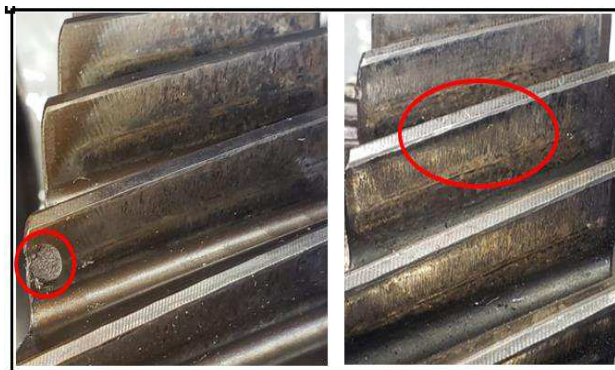
Figure 5 - "Scoring" Destructive Initial.
