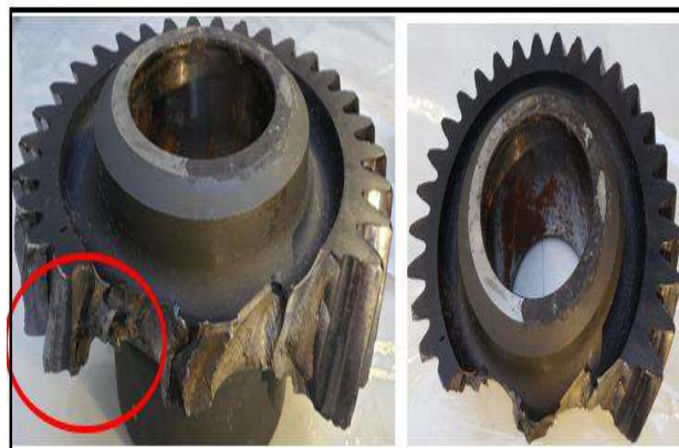
Figure 7 - Impact Break at the Tooth Root.
