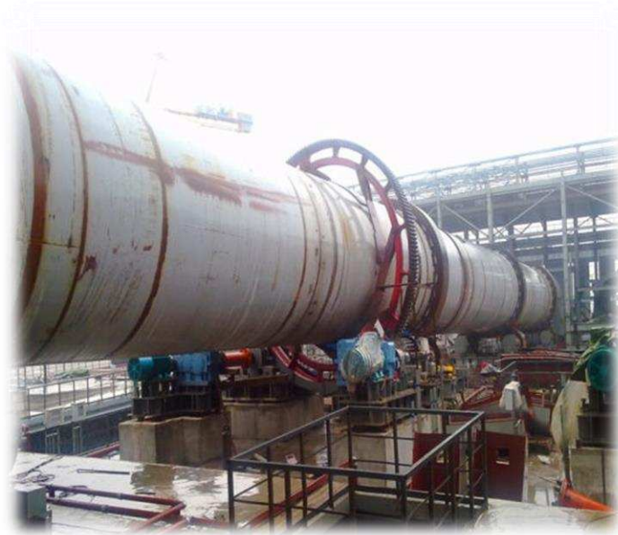
Figura 3. Forno rotativo industrial de grande porte. (Fonte: link.made-in-china.com/co_hnyhks/product_Rotary-Kiln-Furnace-for-Sponge-Iron-Calcination )
