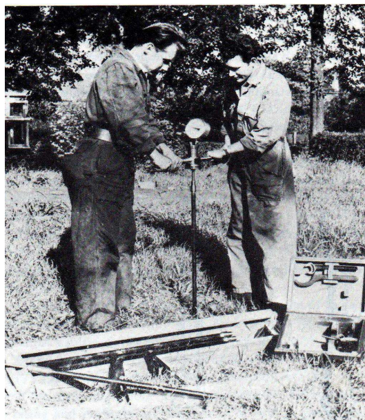
Figura 0.18 - Light-duty Dutch penetrometer (SANGLERAT, 1972)
