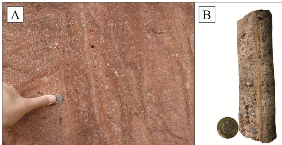
Figure 4.3: Photos corresponding to (A) conglomerate sandstone of fine to clay matrix affected by DB and (B) plug representative of conglomerate sandstone unit of fine to clay matrix
