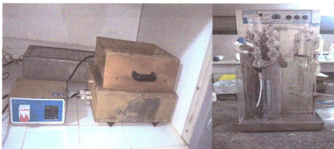
Bloco Digestor (a)
