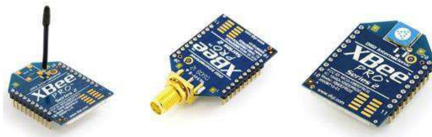
Figura 3. Módulos Xbee-Pro Series 2 [2]
