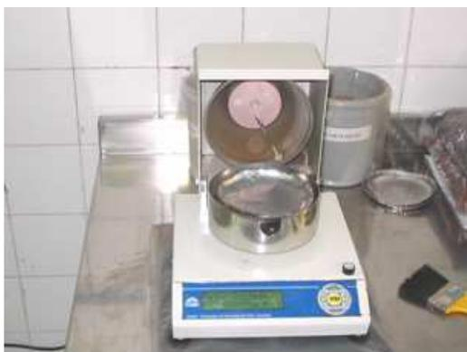
(c) *Medidor de Umidade Infravermelho.*
