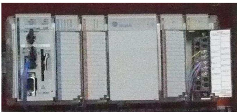
Figura 5.9: CLP CompactLogix.
