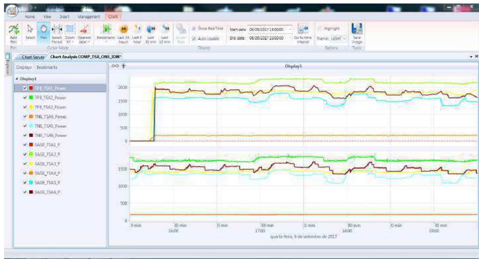
Figura 6.15 – Elipse Plant Manager - Consumo dos Transformadores Auxiliares
