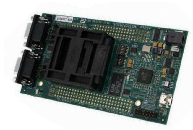
Figura 2.24 – Kit eZdsp TMS 320F28335
