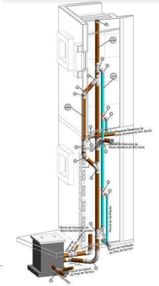
6 DETALHE ISOMÉTRICO SHAFT
