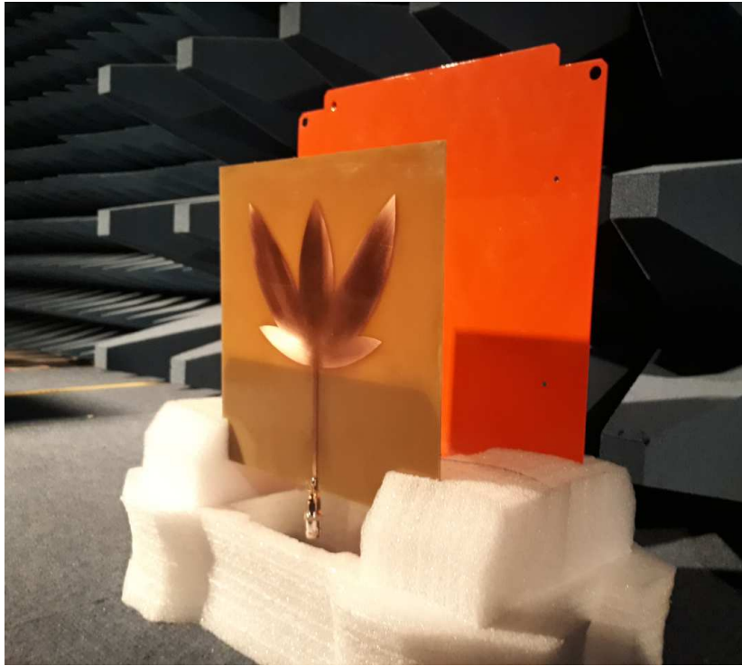
Figure 7. Experimental setup for the electromagnetic shielding test.
