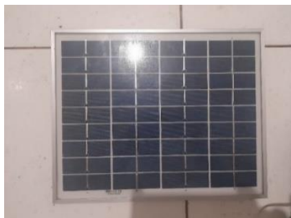
FIGURA 30 - PAINEL SOLAR 10W
