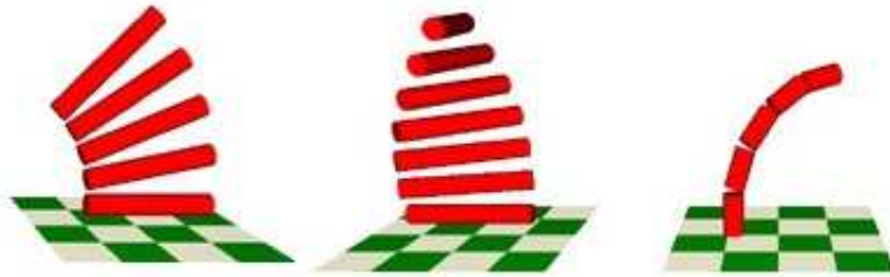
Figura 4.1: K_{11} (Splay), K_{22} (Twist) e K_{33} (Bend)[74].
