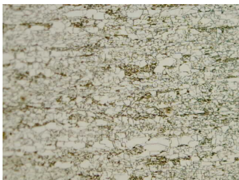
(a) Metal de base – microestrutura unida – 100x
